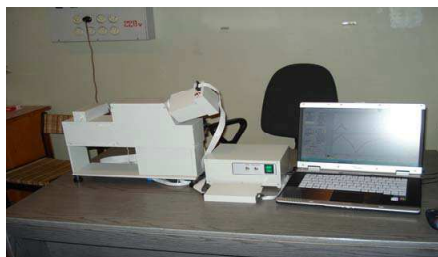
Figure 1: High precision real-time multi-wavelengths spectroellipsometer with binary polarization modulation.
