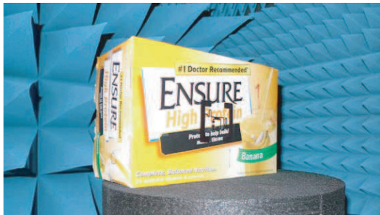
Figure 2: Measurement cabinet and the measured tag on six-pack of cans.
