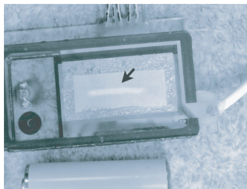
Figure 2: Photograph of prototype FUV plane-emission device in operation. Filament shape of white line indicated by arrow shows far-UV light emission of 1.7 \times 0.16 \text{ cm}^2 . A size-AA dry battery is shown for size comparison.
