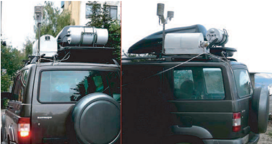
Figure 1: Mobile microwave system installed on UAZ “Patriot”.
