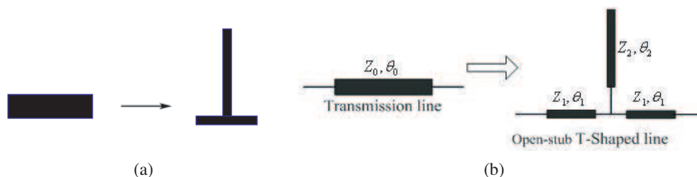
Figure 2: Series transmission line is replaced by open-stub T-shaped. (a) Sketch, (b) equivalent transmission model.
