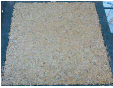
Figure 3: Rice husk particle board.
