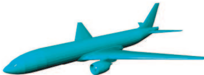
Figure 3: CAD model of the Boeing 777 airplane used in the simulations, length 0.64 m.
