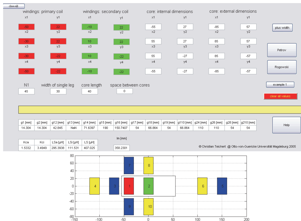
Figure 3. Template of the realized computer program for leakage induction calculation (example for calculation using method of PETROV).
