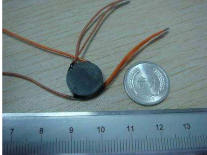
Figure 5: photograph of the piezoelectric transformer with a composite structure.
