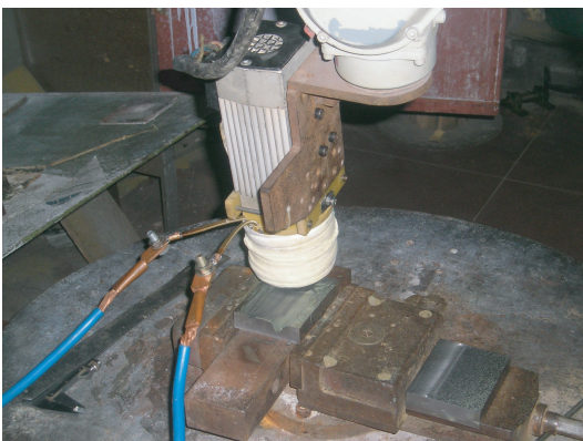
Figure 2: Robotic polishing process with electromagnetic field.
