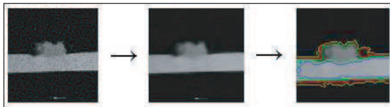
Figure 2: Example of the image processing, from the left: the original image, the wavelet transform filtered image and the segmented cluster by four-phase level set segmentation (green curve).
