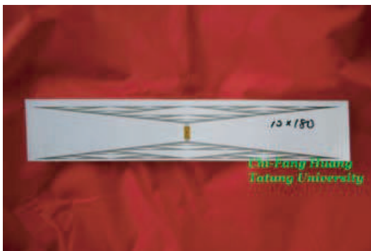
Figure 2: A tag using paper substrate.
