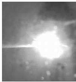
(a) The appearance of the single plasma arc beam (Left: the original arc image. Right: the image figure)
