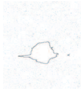
(b) The hybrid arc beam appearance under the condition of average power 4 W (Left: the original image. Right: the image figure)
