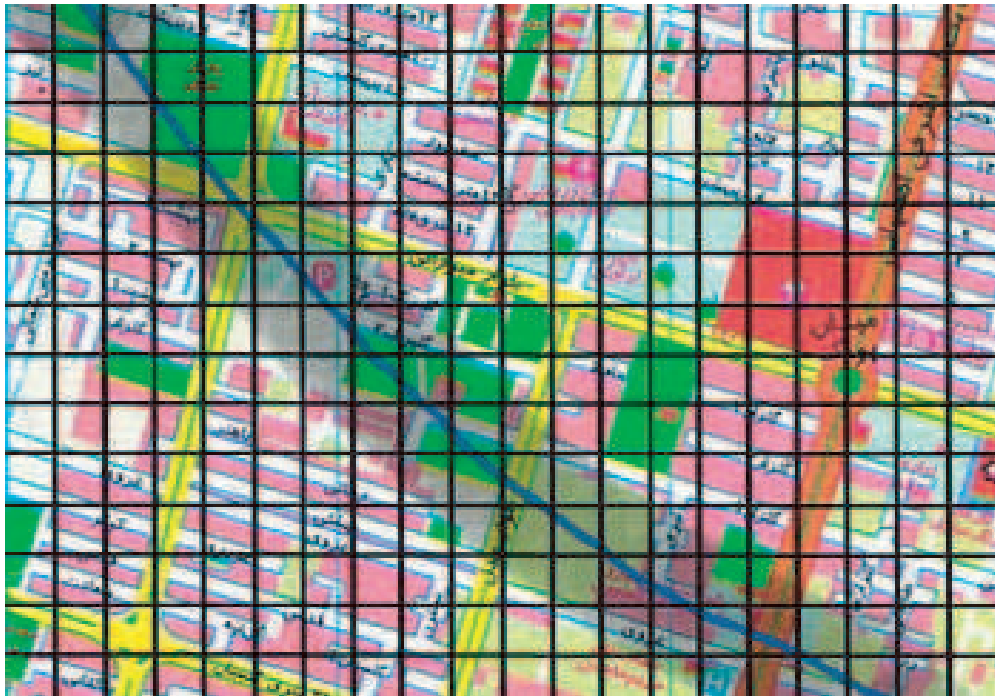
Figure 2: 230 kV power lines transition, in arbitrary region of Tehran (squares size is real). Gray shadow shows the 100 meters border in per side of cable.
