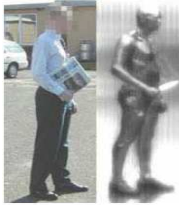
Figure 2: Detection of hidden metal weapons by THz wave.
