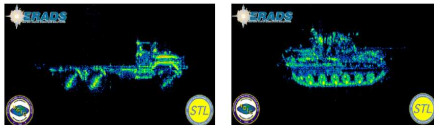
Figure 3: THz radar imaging of military targets.
