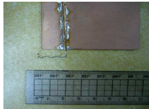
Figure 2: The proposed L-band DVB-H antenna (meander wire monopole type).
