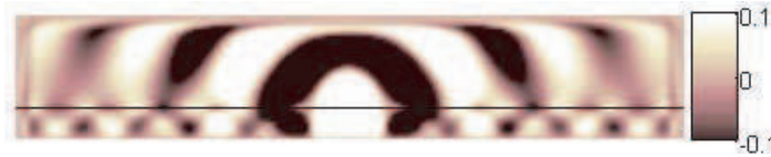
Figure 4: Surface wave cannot be supported by anisotropic grounded slab in Case II. d = 1 cm, \varepsilon_{1y} = (-0.5 - j0.0074)\varepsilon_o , \mu_{1x} = \mu_o , \mu_{1z} = (-1 - j0.0138)\mu_o , \varepsilon_2 = \varepsilon_o , \mu_2 = \mu_o .
