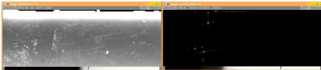
Figure 1: Real L-band clutter (left) obtained by the SETHI airborne radar at L-band, and simulated signal SAR image (right) of 2 point-like reflectors and 1 frequency shifted coded transponder. Red square indicate true ground position of transponder, which appears closer to the aircraft and blurred.
