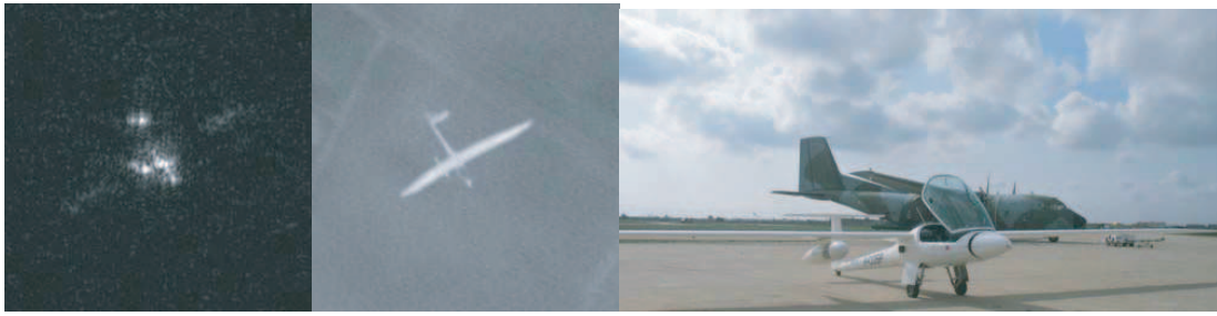
Figure 8: In flight SAR image (left) and optical image (middle) of the receiver aircraft, a Stemme touring motor glider, with a T shaped tail and the receiving radar under the right wing. Photo (right) on the ground of the receiver aircraft with the illuminating aircraft on the background.
