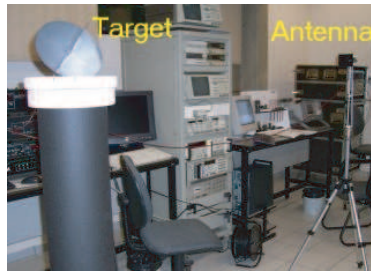
Figure 1: Antenna, target and associated electronic equipment of the Lab-Volt Training System. The target rests on a cylindrical styrofoam pedestal.
