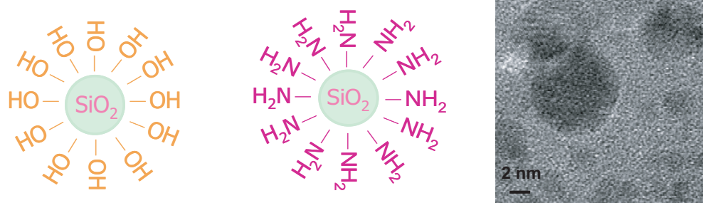
Figure 2: The schematic molecular structures of the studied HPND and APND also shown is the TEM image of the HPND.
