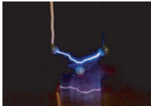
Figure 3: Electric discharge from positive and negative electrodes to a mesa-type lead placed at a cusp center on a copper plate. Above bright light is a real discharge, while lower weak light is its image. The voltages of electrodes are \pm 21 KV both and discharge current is around 590 \mu\text{A} . The mesa diameter is 5 mm. It is interesting to compare flat discharge to mesa-type object with sharp discharge to hemisphere in Fig. 4. Also, neither direct discharge between two electrodes nor electrodes to copper ground occurred because of more electric field merging from both electrodes to object.
