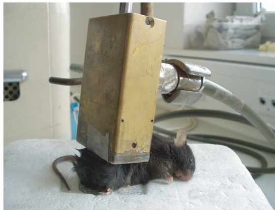
Figure 1: Waveguide applicator for biological experiments.
