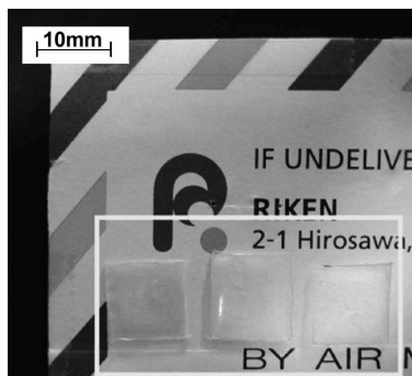
Figure 1: View of the samples. The small polyethylene bags contain from left to right: MDMA, aspirin, and methamphetamine. The bags were placed inside the envelope during imaging. The area indicated by the white line represents the imaging target, 20 \times 38 mm in size. Since methamphetamine and aspirin are similar in appearance, we used a slightly longer bag for the latter to avoid confusion.
