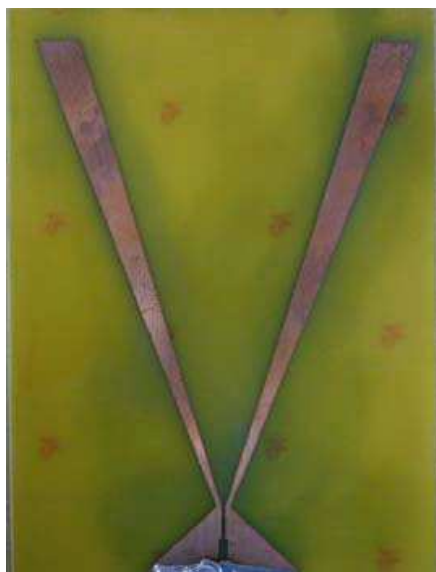
Figure 1: V-dipole antenna fed by Marchand balun.
