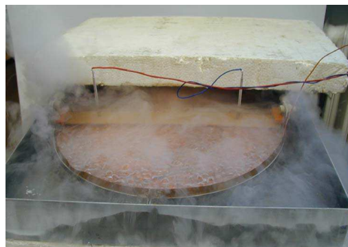
Figure 6: The dependence of electric conductivity \gamma on temperature: The measurement configuration.
