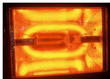
Figure 13: Induction neon lamp with the power of 500 W.
