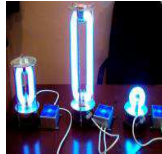
Figure 7: Pilot samples of electrodeless amalgam UV lamps with the power of 100, 200 and 50 W (from the left to the right).
