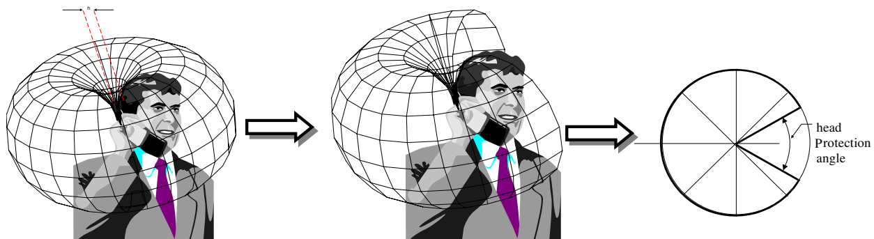
Figure 1: Requirements for antenna radiation pattern.
